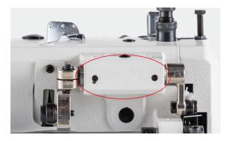
**5**Sealed presser foot lifter shaft,no oil, no trouble
